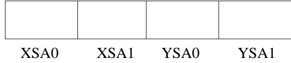
Figure 1: The MMA composite signature for node X bridged to node Y is the union of the four stuck-at signatures for the two bridged nodes. Each stuck-at signature is a set of output:vector pairs.
