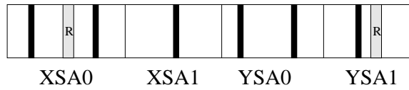
Figure 3: The composite signature of X bridged to Y with match restrictions (in black) and match requirements (labeled R)
